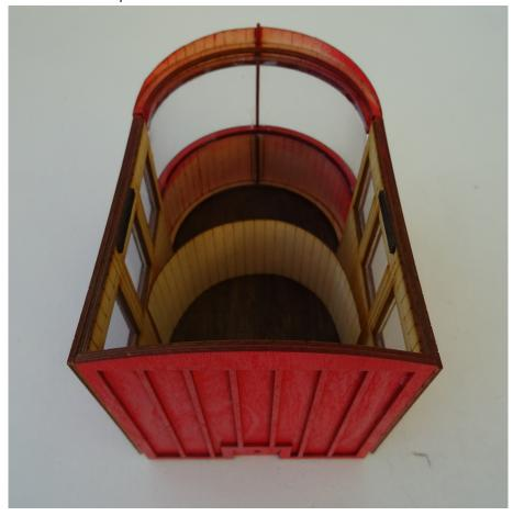
If you have not fitted the inner side skins and windows now is a good time to fit them. The windows and glazing should be fitted next, glazing inside window frame outside. They are a tight fit so that they cannot move out of alignment.
